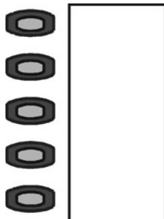
The **function keys** next to the lettering label are programmable keys, e.g. to assign speed dial numbers or operate telephone functions. The LED shows the status of the function.
