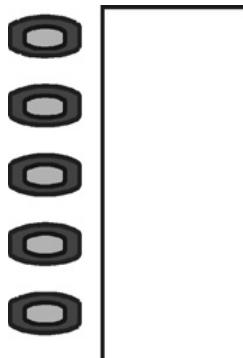
The **function keys** next to the lettering label are freely programmable keys, e.g. to assign speed dial numbers or operate telephone functions. Each key has two levels that can be assigned functions.
